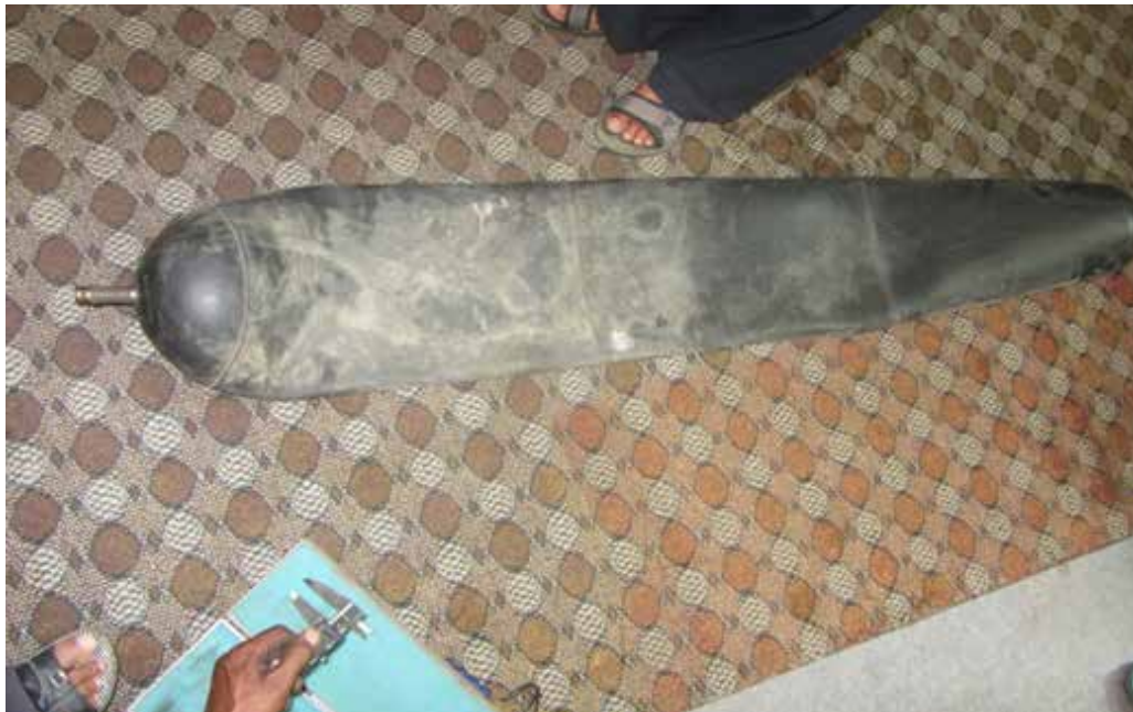
Replaced bladder of OPU in Unit I & Unit II, 2076
