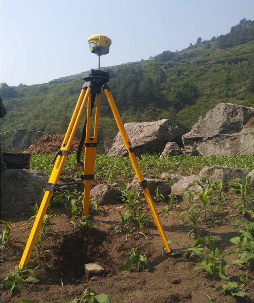
DGPS observation at Nyak with reference to National Geodetic Control Points
