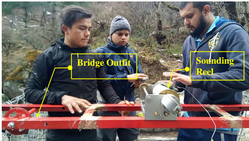
Setup of current meter for discharge measurement
