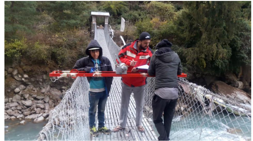
Discharge Measurement of Budhi Gandaki River at headworks
