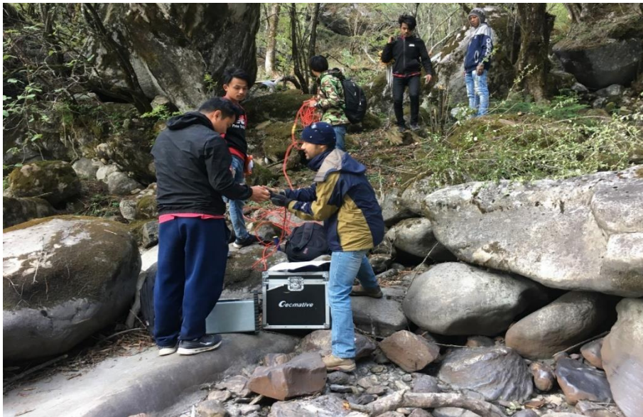
Laying of electrodes and acquisition of data during ERT survey
