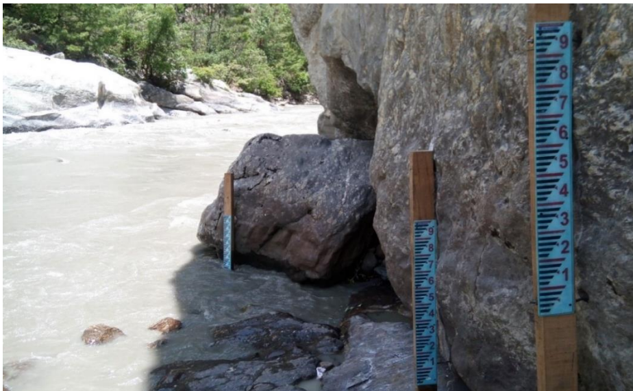
Installed gauge installation at downstream of confluence (Budhi Gandaki Rier and Tom khola
